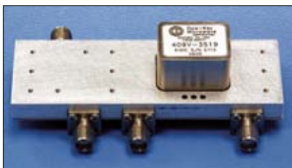
Fig. 1 The 409 switch mounted in a PCB fixture.
